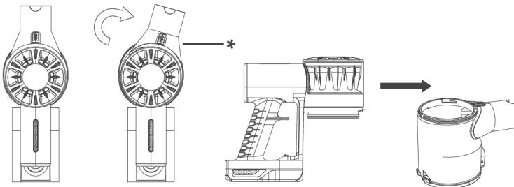
To release the metal filter from the motor unit, turn it to the left.
