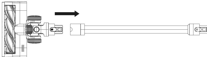
To remove, press the release button and detach.
