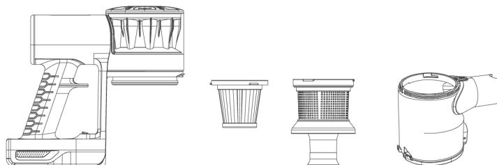
Wash the container and filters with water. Do not use solvents, acidic or basic cleaning agents like bleach, or abrasive products, as they may damage the components.
