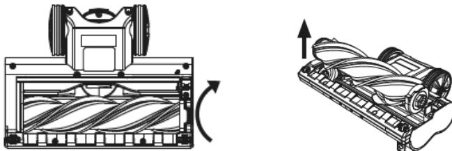
To remove the rotating brush, release the side latch of the motorized brush.
