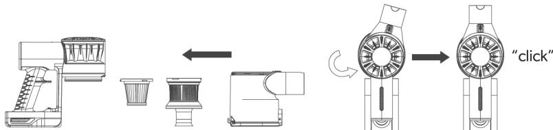
Reattach the dust container, ensuring the bottom part fits securely onto the motor unit.
